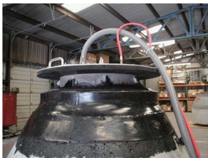
Riser-Wrap™ Vacuum Test
